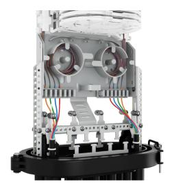
FOBP-R fiber optic closure has also the new design of mounting SCM-C splice trays. The installation is performed by inserting trays into a holder. Consequently, all these changes made installation of oval splice trays easier, faster and less exposed to damage during installation and operation.
